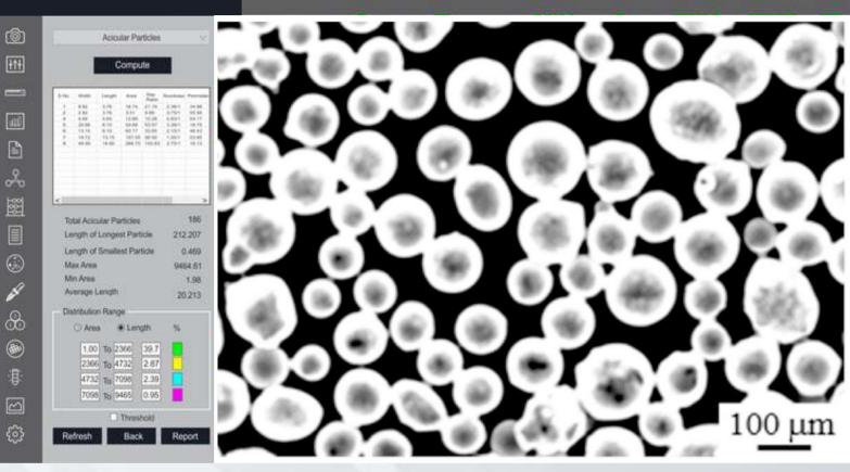
Particle Size & Shape Analysis Software - Particle Size Soft
